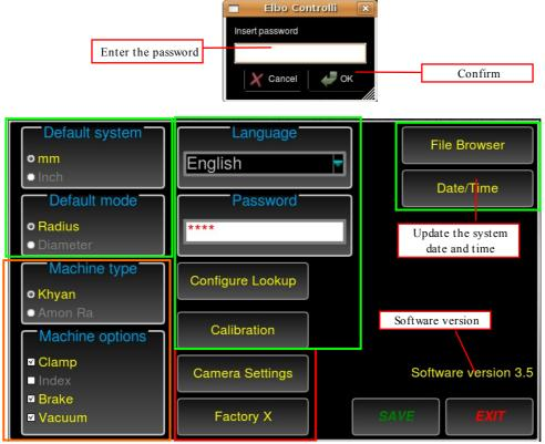
Figure 19: Software configuration
