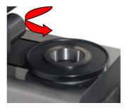
• Introduce the tool and press the key to perform the clamp: the following screen will be displayed and it will ask you to rotate the spindle holder in clockwise direction.
