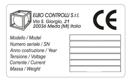
The relevant information for each specific machine is summarized on the identification plate (illustrated above) displayed on the left side of the presetter.
