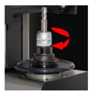
• After a few revolutions, you will notice a resistance in the rotation and after that a click; after the click, the rotation of the spindle holder will be free again and a screen will be displayed to specify that the clamp was performed in a correct way.
