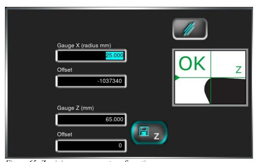
Figure 65: Z origin measurement confirmation
