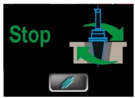
• To remove the tool, press the unclamp key once more, and then rotate the spindle holder in counter clockwise direction until completely releasing the same tool, as specified in the picture that is shown in the display.
