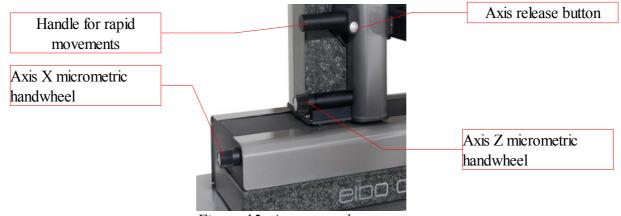
Figure 15: Axes control
