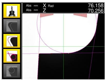
Figure 35: Automatic geometry calculation
