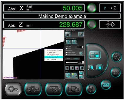
Figure 49: Chamfer measurement
