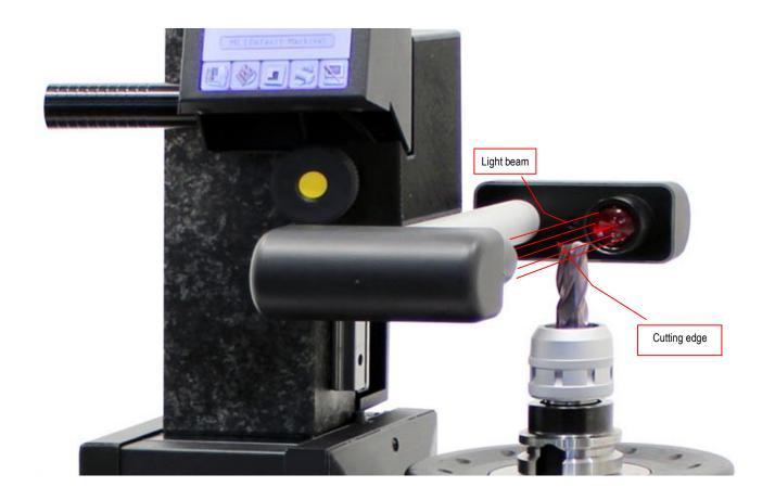
The focusing control bars supply information about image sharpness in the measurement points that are specified in the figure; therefore, it's possible to obtain different pieces of information (in the maximum value) for different tools or also for different cutting edges in the same tool. For example, this depends on the ware level or the relief angle.
