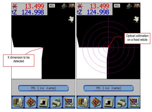
In these cases, measurement needs to be manually carried out, by using the device as a normal profile detector.
