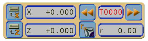
For each tool it's possible to be memorized: the letter "**T**" of the corrector used by the numerical control of the machine(from 1 to 9999), the "**X**" and "**Z**" dimensions and the radius "**r**".
