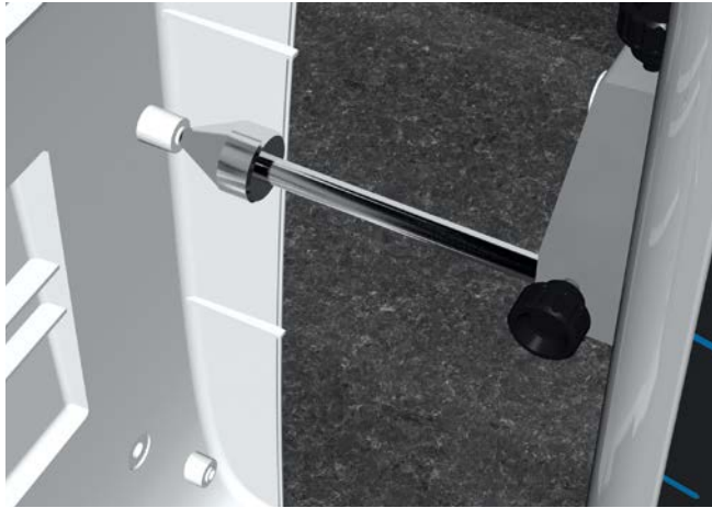
Measuring centre distances on a plastic casing of an electronic box
