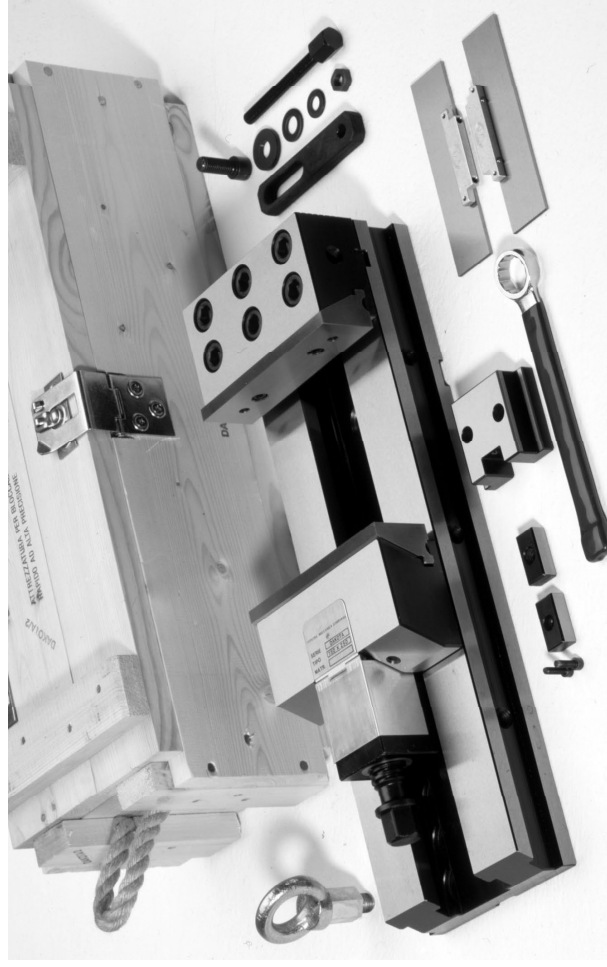
Clamping equipment Tct complete with wrench, work stop, rigid slide way, floating slide-way (for raw work-piece), pair of positioning keys, pair of CLAK parallels, cover for the protection of the screw, eye bolt for lifting, wooden packing case.
